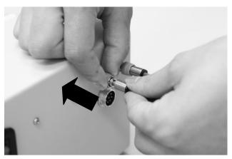
4. As shown in the picture below, release the lock to remove the grey cable.
